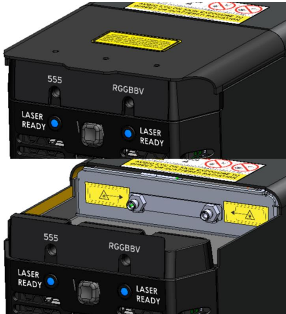
Figure 10. Top: LDI with the fiber access cover. Bottom: LDI without the fiber access cover.
