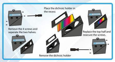
To fit your dichroic mirror into the Cairn Filter Cube remove each of the four screws that secure the two halves together. You will then be able to gently pull the two halves apart. There is one steel locating rod in each half of the cube to ensure the correct alignment when it is reassembled. Once the two halves of the cube are seperated place the dichroic mirror (active side down) into the rectangular recess. Then simply reassemble the cube and tighten the screws.
