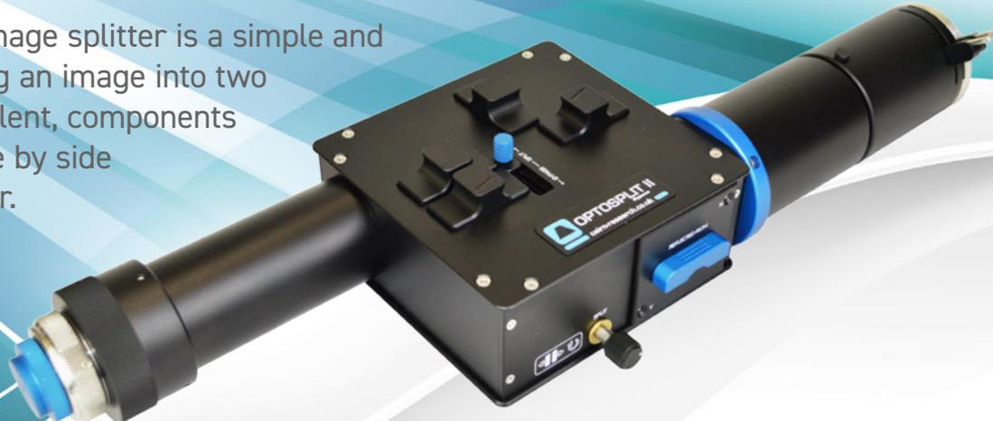
The Cairn OptoSplit II BP is our best ever dual channel simultaneous imaging device for use with a single camera. It builds on the success of the OptoSplit II, but adds a convenient single lever bypass mode making it more suitable for multi-user microscopes where simultaneous dual channels are only required for specific experiments alongside single wavelength recordings.
