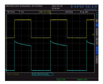
The yellow trace shows a pulsed current going through the LED, and the blue trace is the optical output, for a 505nm and 590nm LED respectively. The timescale is 5msec per division. One can see that in both cases the optical output declines during the "on" period. The effect isn't too bad for the 505nm LED, but for the 590nm one it's quite serious. So what is going on here?
